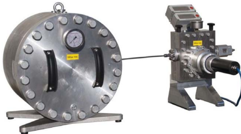
Figure 2. Equipment to float optical fibers into steel tubes. Left: fiber pay-off in pressure tank, Right: dividable pressure housing injecting the water into the steel tube and mechanically advancing the fiber.
