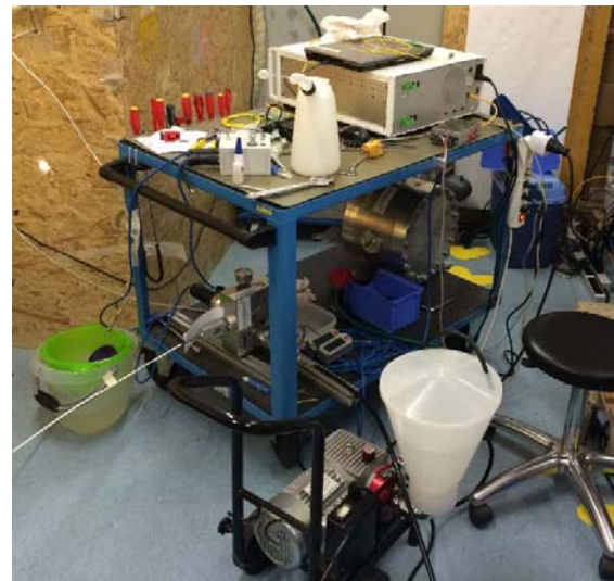
Figure 5. Floating 485 \mu\text{m} fiber into 3.18/2.16 m steel tube. Big pressure tank used. 3 km with 90 bar.
