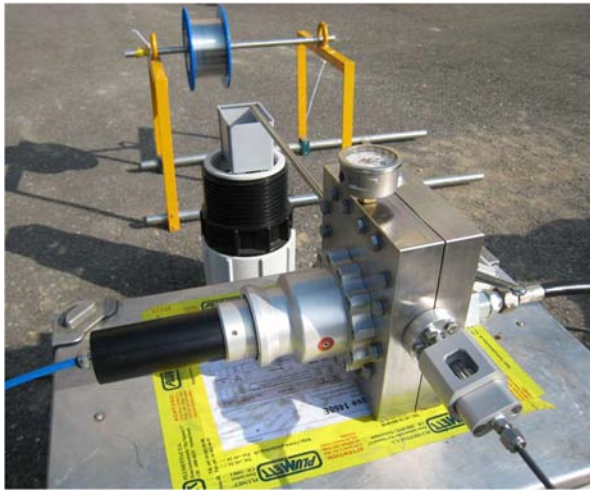
Figure 3. Floating 250 \mu\text{m} fiber into 4.76/2.76 m steel tube. No pressure tank used. Here with alcohol.
